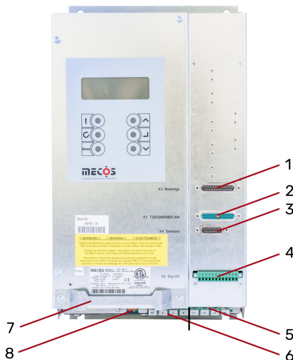
Figure 7: Front view of inverter & magnetic bearing electronics MMC15
